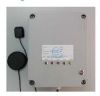
The position data acquired by the *uH-5i* are communicated via the both GSM (GPRS/SMS) & Iridium satellite networks to a Central Monitoring Station located at the management office of the user that logs and process the incoming position data to display on the monitoring software.
